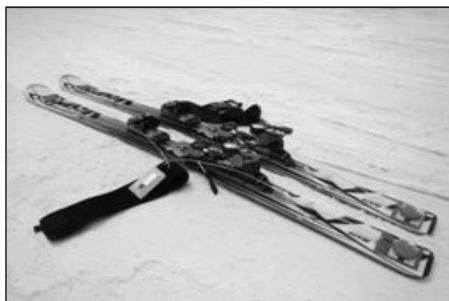
Figure 5: Ski with two transmitters on both ends of the ski
